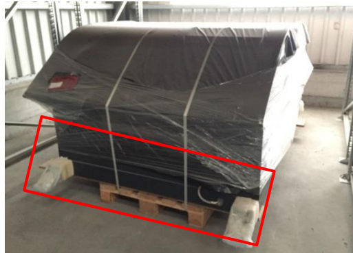
Figure 2 Example of an incorrect load unit
