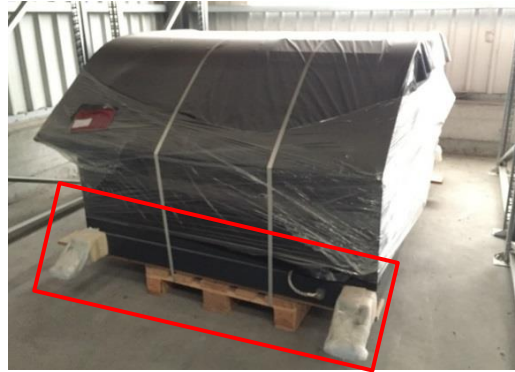
Figure 3 Example of an incorrect load unit
