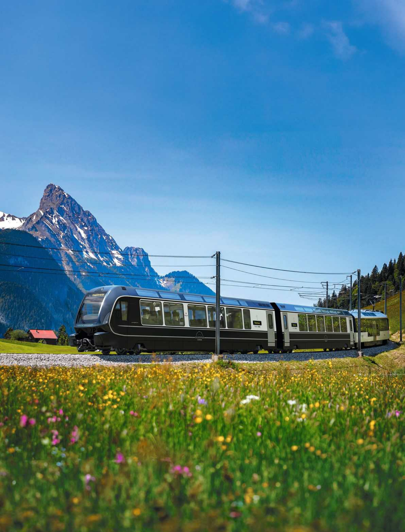
The GoldenPass Express has bogies with adjustable wheel sets and can therefore run on both narrow-gauge and standard-gauge tracks. It was named the most beautiful train in the world by National Geographic in 2023.
