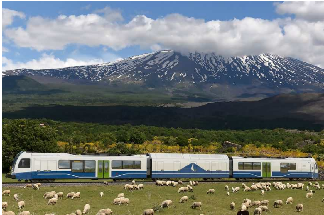
The new hydrogen trains for Sicily are expected to run along the Etna Nature Park from 2028. Each vehicle consists of two passenger cars and a central “Power Pack”, which contains elements such as the water tank.
