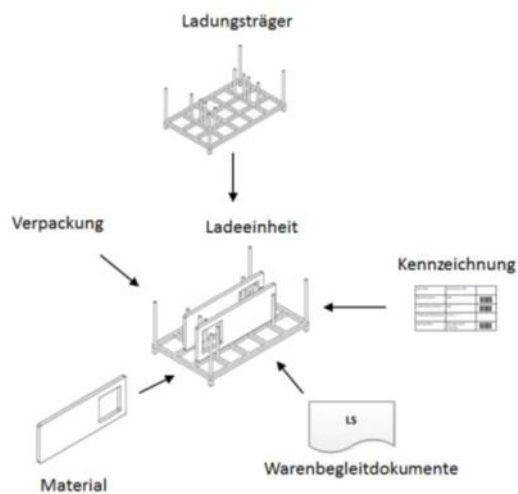
Figure 7: Creation of a load unit for delivery variant 3
